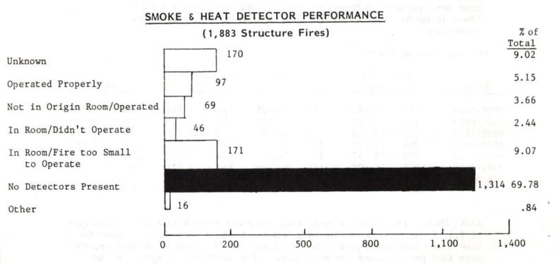
ANALYSIS: Of the detectors that are installed, we had a fair success rate: Known installations 383 versus only 46 known failures; 88% success. What is a startling statistic is there are still many properties with no
