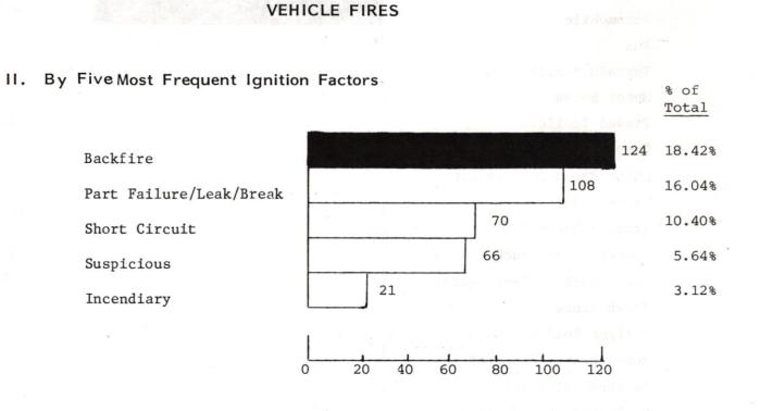
ANALYSIS: The leading category is backfire and this is generally cured by a tune-up. Also, it has been my experience that most backfire vehicle fires do not have an air cleaner on the carburetor.
